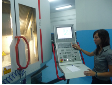
(a) Machining/ Milling Center of HERMLE type-C 20 U (iTNC 530)
