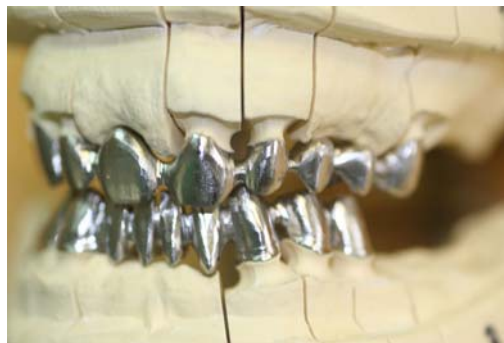
Fig. 1. Metal pieces manufactured by a dynamic high-precision machining centre with five axes
