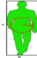
Fig. 4. Influence Radius of a track while using the Optical Flux Method
