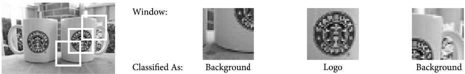
Fig. 3. An overview of the sliding window method, where an input image is subdivided into smaller overlapping image patches, each being individually analyzed by a CNN
