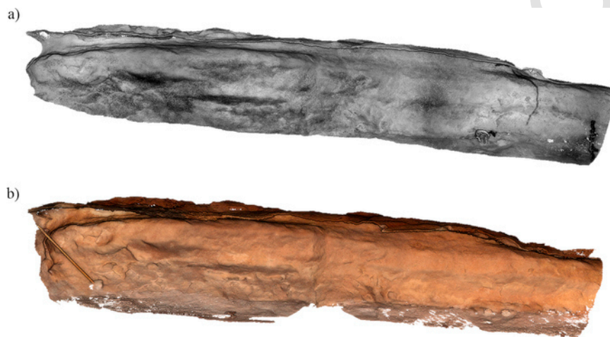
Fig. 4. Graphical comparison between point clouds: (a) coming from TLS; and (b) coming from digital camera.
