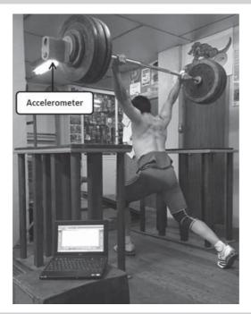
Figure 1. Weightlifter perform the lift with the accelerometer fixed to the bar according to the study by Sato et al. (29).
