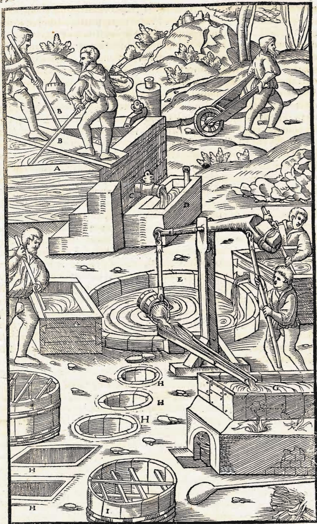
At saxa aluminosa primò in fornace calcariæ simili sic urantur. In fundo fornacis ex id genus saxis fiat testudo: quæ sit ignis receptaculû: reliqua fornacia
