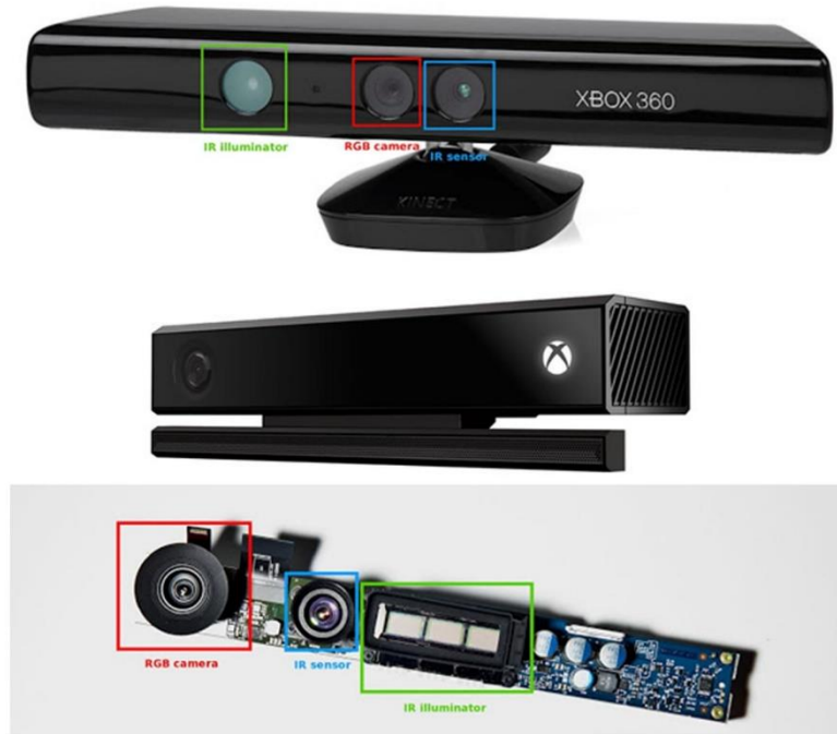
Fig. 1. Kinect I laser scanner with highlighting of IR illuminator, RGB camera and IR sensor (top), and Kinect II laser scanner with RGB camera, IR sensor and IR illuminator (bottom).
