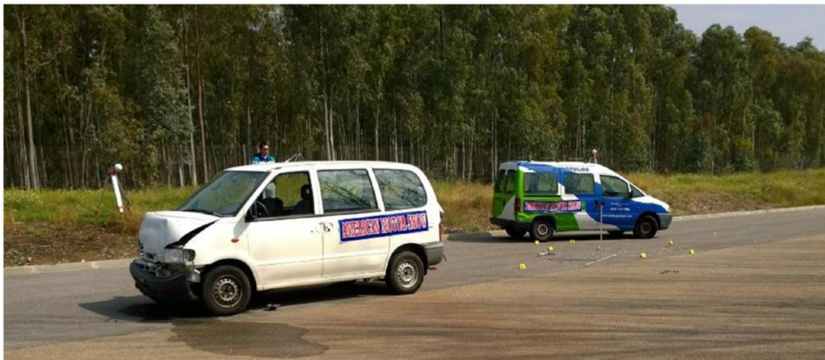
**Figure 4.** Final position of the crashed vehicles involved in the simulated accident. It can be appreciated (between both cars) the metallic scale bar used for providing metric capabilities to the photogrammetric reconstruction.
