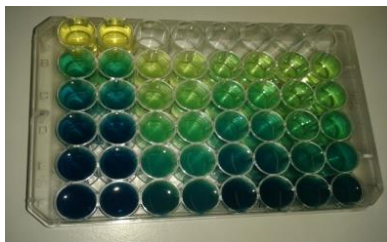
Figure 14. Multiwell plate showing samples prepared for measurement of the reducing power assay. The stronger the antioxidant concentrations the darker the Prussian blue tone.
