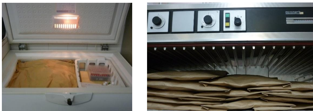
Figure 8. Processing of stevia samples: left photo, frozen at -20 °C; right photo, dried-oven at 30 °C.
