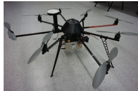
FIGURE 2: Aerial 3D Mapping System developed.
