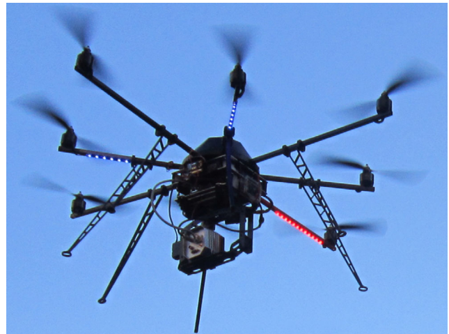
Fig. 1. UAV equipped with thermographic camera.
