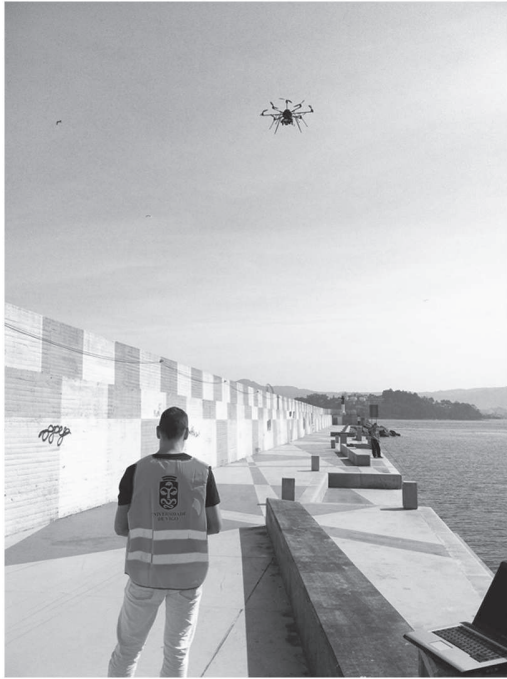
Fig. 2. Mikrokopter UAV with Sony Nex 7 during survey (image by Higinio González-Jorge)
