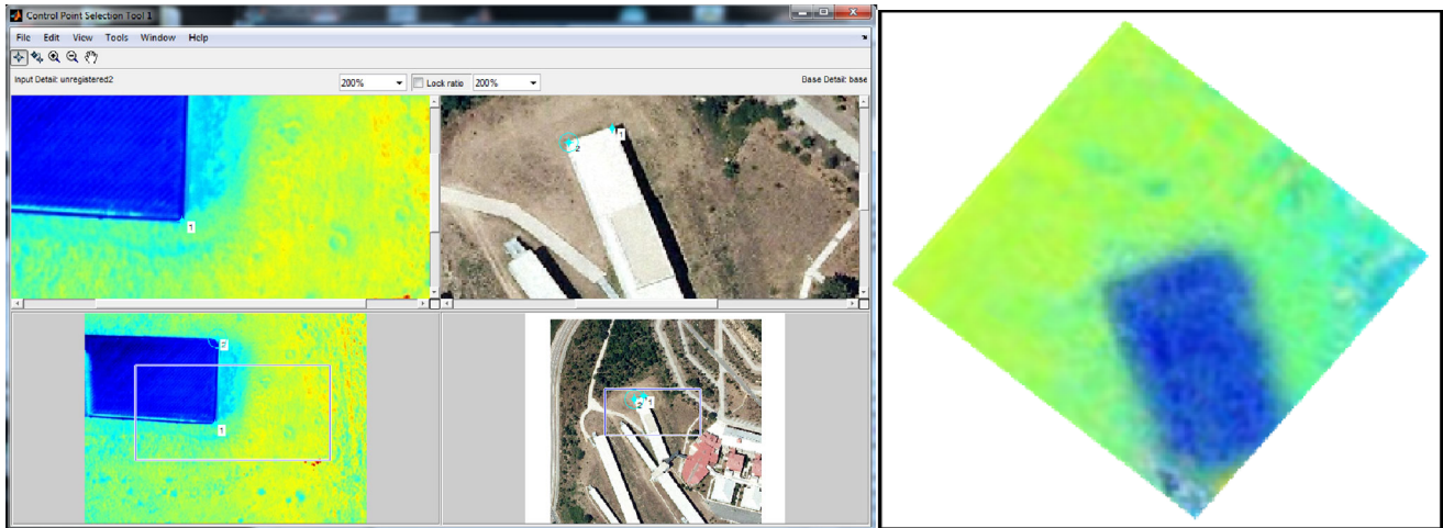
Fig. 4. Image registration process (left); registered image (right).
