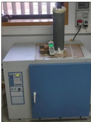
Figure 8. Equipment designed to measure thermal conductivities.
