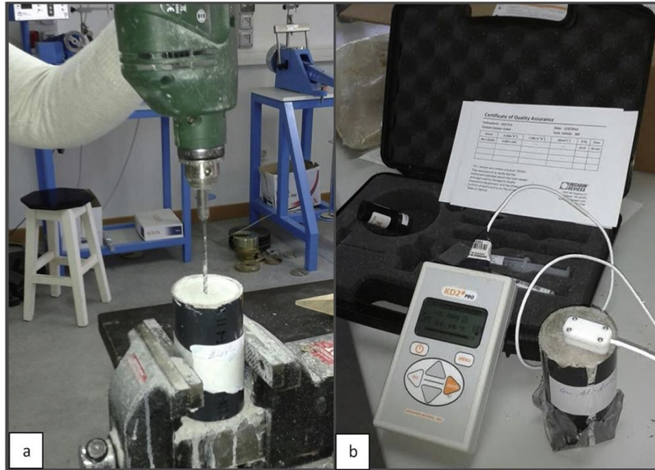
Fig. 4. (a) Drilling of a hole to insert sensor RK-1. (b) Measuring of thermal conductivity with equipment KD2 Pro.
