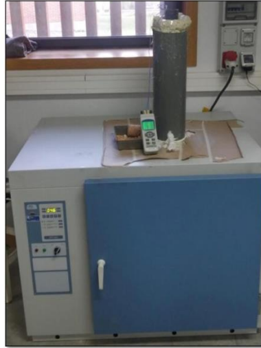
Figure 8. Equipment designed to measure thermal conductivities.
