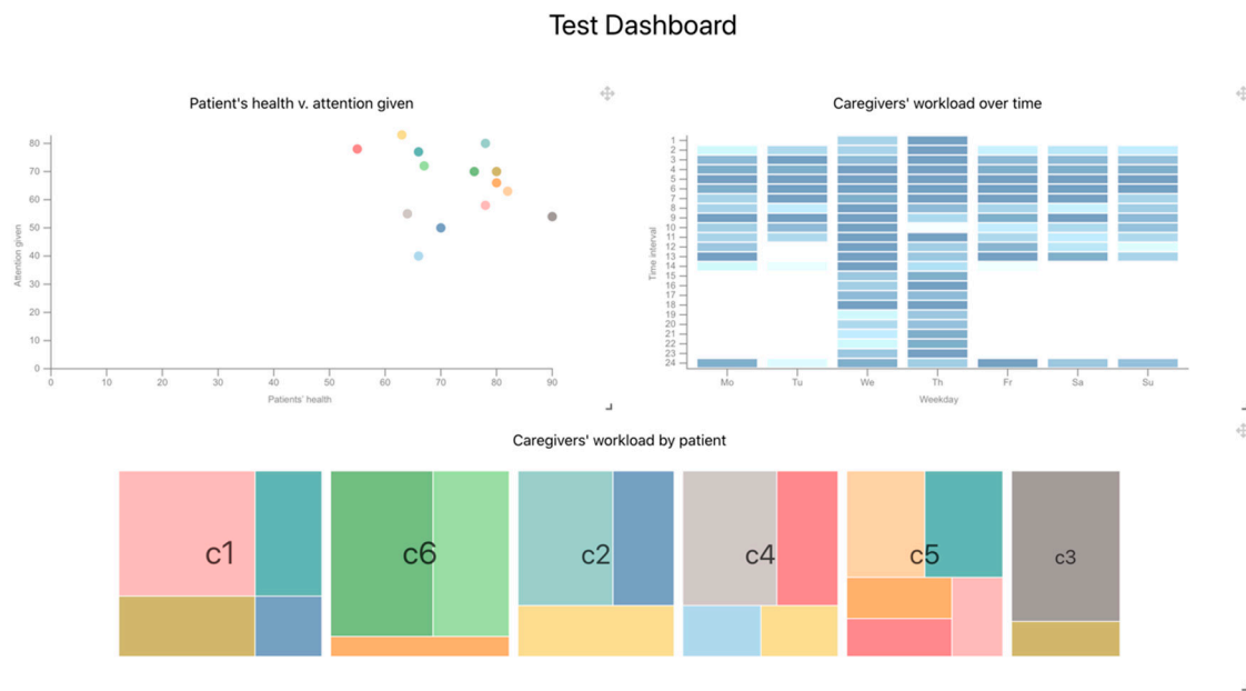
Figure 10. Screenshot of the dashboard generated through the XMI instance. Three visualizations are shown: a scatter plot that display potential relationships between the patients' health and the attention given to them; a heatmap that display the aggregated workload of the caregivers during the different days and hours of the week; and a treemap that display the individual workload of each caregiver.
