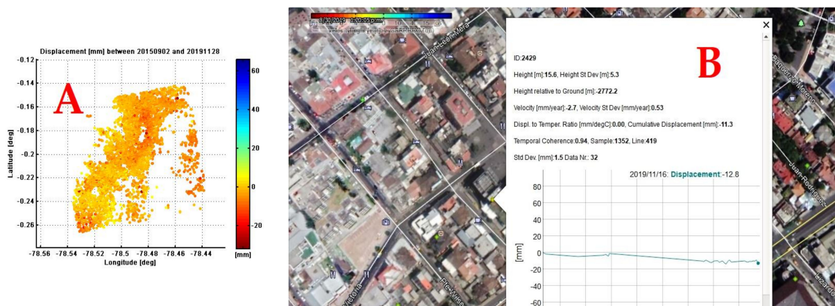
Figure 7. (A) Scatter plots of velocity for each point of the area. (B) Multi-time displacement and velocity analysis (2015–2019 series).
