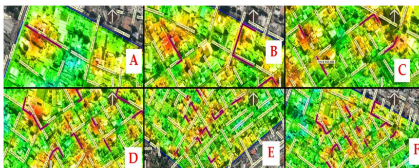
Figure 14. Escape routes near the areas of greatest exposure that the population can reach in a very short time between 1 and 4 min (red-black double line routes in the figures from A–F).
