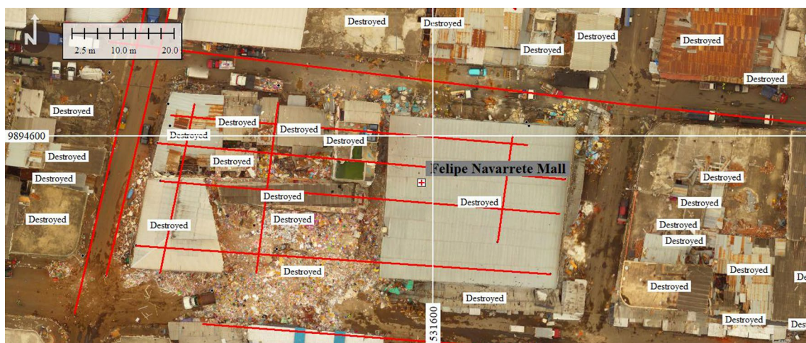
Fig. 9 Location of the network of geophysical research lines, electrical tomography and georadar in the areas of maximum deformation of the ground, for the investigation of the subsoil. In the same line of
