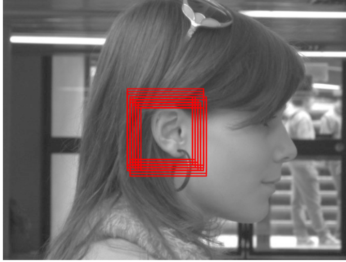
Figure 6.3: Sample of multiple overlapping detections casted as individual detection windows on an input image.
