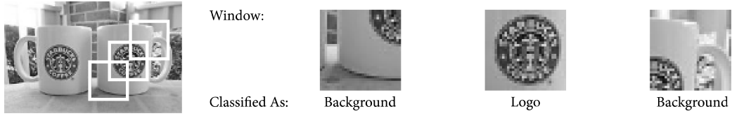
Figure 3.14: An overview of the sliding window method, where an input image is subdivided into smaller overlapping image patches, each being individually analyzed by a CNN. A classification result is then obtained for each individual window.
