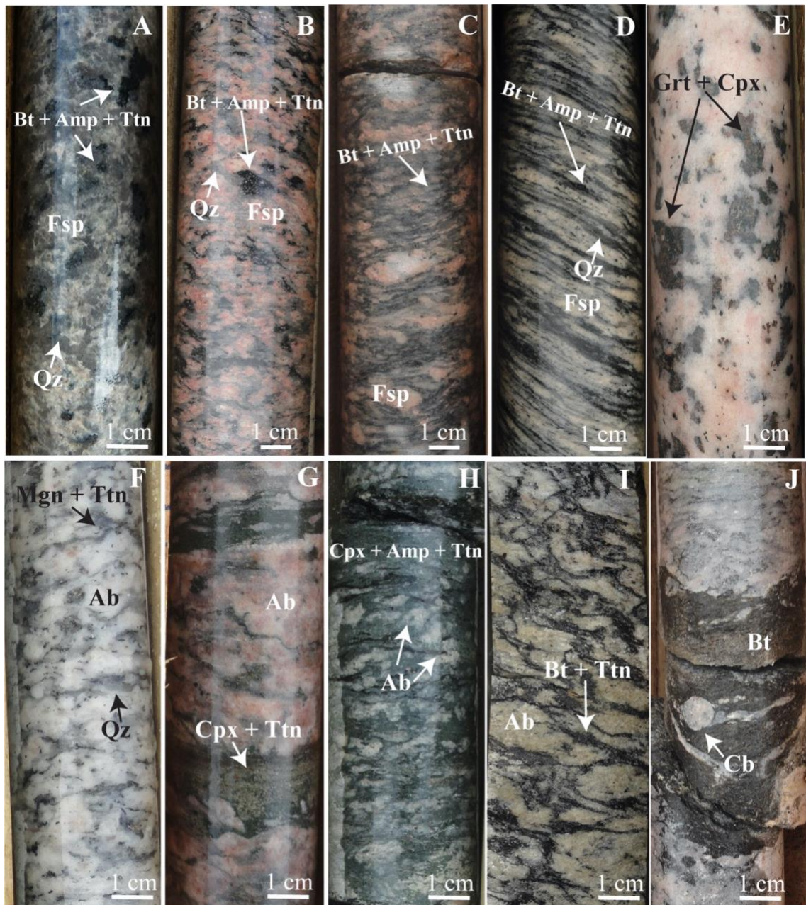
Fig. 20. Drill-core photographs of hydrothermally unaltered to altered rocks at Gameleira I, Barrinha and Barreiro deposits. A. Preserved unaltered and undeformed São Timóteo granite typically coarse-grained and grey in color. B. Weakly deformed São Timóteo granite with a discontinuous foliation showing signs of albitization represented by the pinkish color. C. São Timóteo gneiss showing augen-fabric and a pinkish color as a result of albitization. D. Striped São Timóteo gneiss with stretched crystals of feldspar and quartz. E. Massive garnet-rich albitite with andradite surrounded by Cpx II. F. Magnetite-rich albitite with low mafic contents. Magnetite and titanite are displaced mostly along the foliation. G. Cpx III and titanite concentrated in albitite portions. H. Cpx III \pm amphibole II well developed in an augen-like albitite. I. Biotite-rich augen albitite
