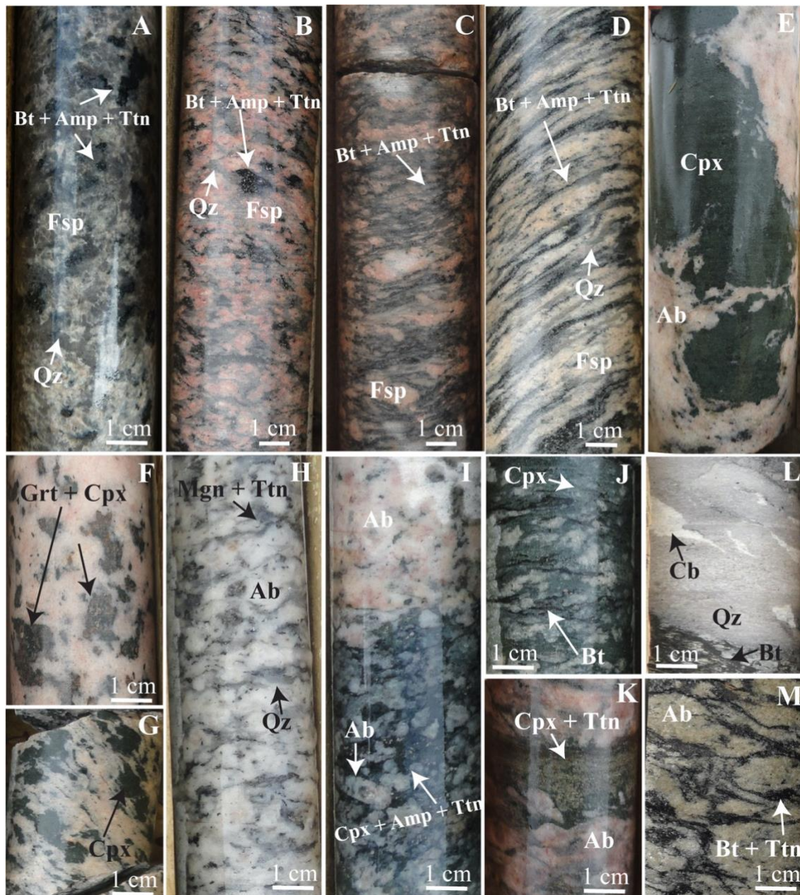
Fig. 45: Drill-core photographs of fresh to hydrothermally altered rocks at the Gameleira I, Barrinha and Barreiro deposits. A. Preserved unaltered and undeformed São Timóteo granite typically coarse-grained and grey in color. B. Weakly deformed São Timóteo granite with a discontinuous foliation showing signs of albitization represented by the pinkish color. C. São Timóteo gneiss showing augen-fabric and a pinkish color as a result of albitization. D. Striped São Timóteo gneiss with stretched crystals of feldspar and quartz. E. Massive pyroxene-andradite bearing albitite. Note the extreme pyroxene enrichment with no apparent fabric. F. Massive pyroxene-andradite bearing albitite, with garnet surrounded by pyroxene. G. Foliated pyroxene-andradite bearing albitite, where the modal volume of pyroxene is enhanced. H. Magnetite-rich albitite with low mafic content. Magnetite and titanite are
