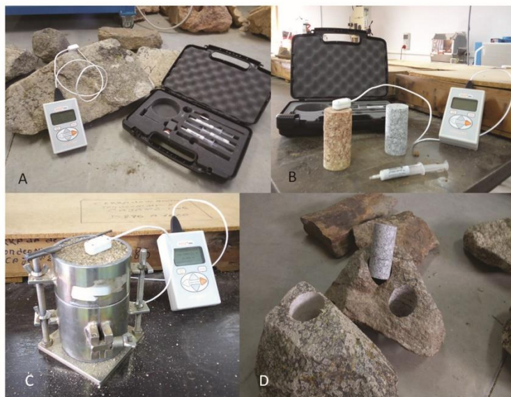
Fig. 2. A) KD2 Pro, (Decagon Devices, 2016) and sensor RK-1. (Range from 0.1 to 6 W/mK, accuracy 10%) B) Rock cores, 5 × 11.5 cm. We must drill to insert the needle (3.5 mm in diameter and 6 cm in length) and use thermal grease to improve the thermal contact C) Proctor compacted soil samples, (in situ water content preserved). D) Core samples extraction.
