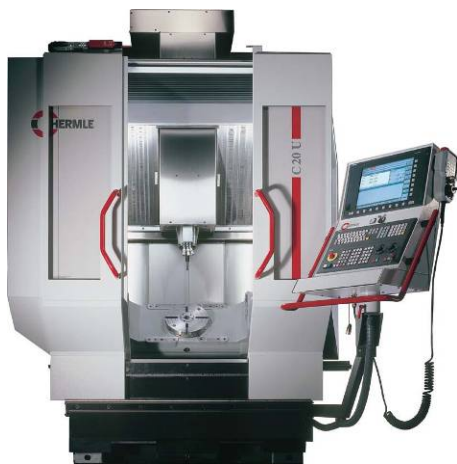
Fig. 5 Machining/ Milling Center of HERMLE type-C 20 U (iTNC 530), with swivelling rotary (280 mm), with a control system using drills and bits of high precision
