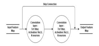
Figure 1. Dataflow diagram of basic block.
