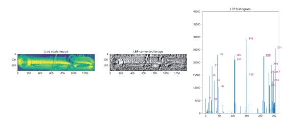
Fig. 9. Grey scale image, LBP Converted image and Histogram of Friction Stir Welded joint (6061-T6 on retreating side) obtained at the tool rotational speed of 800 rpm and tool traverse speed of 800 mm/min.
