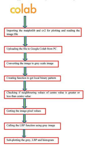
Fig. 7. Steps taken for obtaining the grey image, LBP and histogram of the Friction Stir Welded joint.
