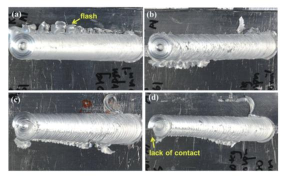
Fig. 6. Friction Stir Welded joints obtained at a constant rotational speed of 800 rpm and varying traverse speeds of 400, 600, 800, 1000 mm/min [13].
