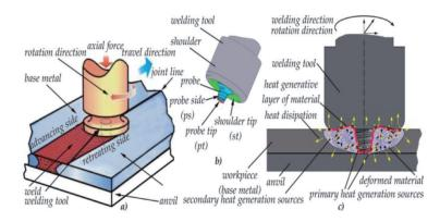
*Fig. 3. a) Friction Stir Welding Setup, b) Tool Nomenclature, c) Heat generation and plastic deformation in FSW process [5].*
