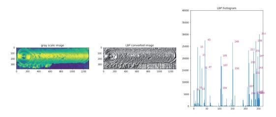
Fig. 8. Grey scale image, LBP Converted image and Histogram of Friction Stir Welded joint (6061-T6 on advancing side) obtained at the tool rotational speed of 800 rpm and tool traverse speed of 600 mm/min.
