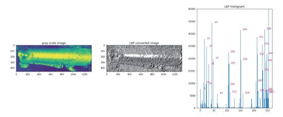
Fig. 8. Grey scale image, LBP Converted image and Histogram of Friction Stir Welded joint (6061-T6 on advancing side) obtained at the tool rotational speed of 800 rpm and tool traverse speed of 800 mm/min.
