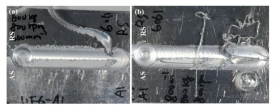
Fig. 5. Friction Stir Welded joints obtained at a constant tool rotational speed of 800 rpm and tool traverse speeds of 600 mm/min and 800 mm/min [13].
