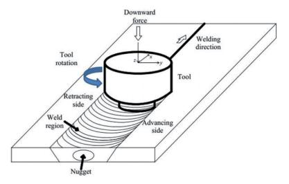
Fig. 2. Mechanism of Friction Stir Welding process [3].
