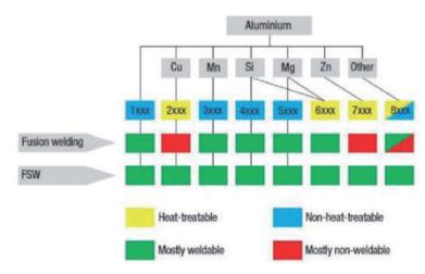
Fig. 1. Comparison of the weldability of different aluminium alloys by conventional and Friction Stir Welding process [2].
