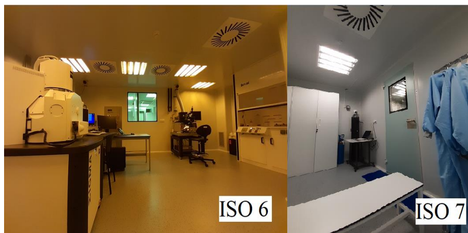
Figure 3: The lithography room and dressing room of the University of Salamanca cleanroom, belonging to ISO 6 and ISO 7, respectively.
