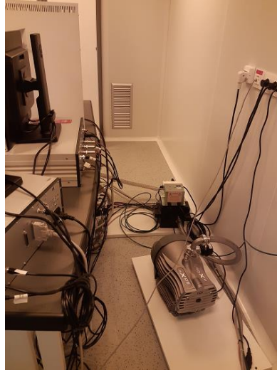
Figure 8: A scroll pump is used as a backing pump of a turbomolecular pump for the scanning electron microscope equipment.
