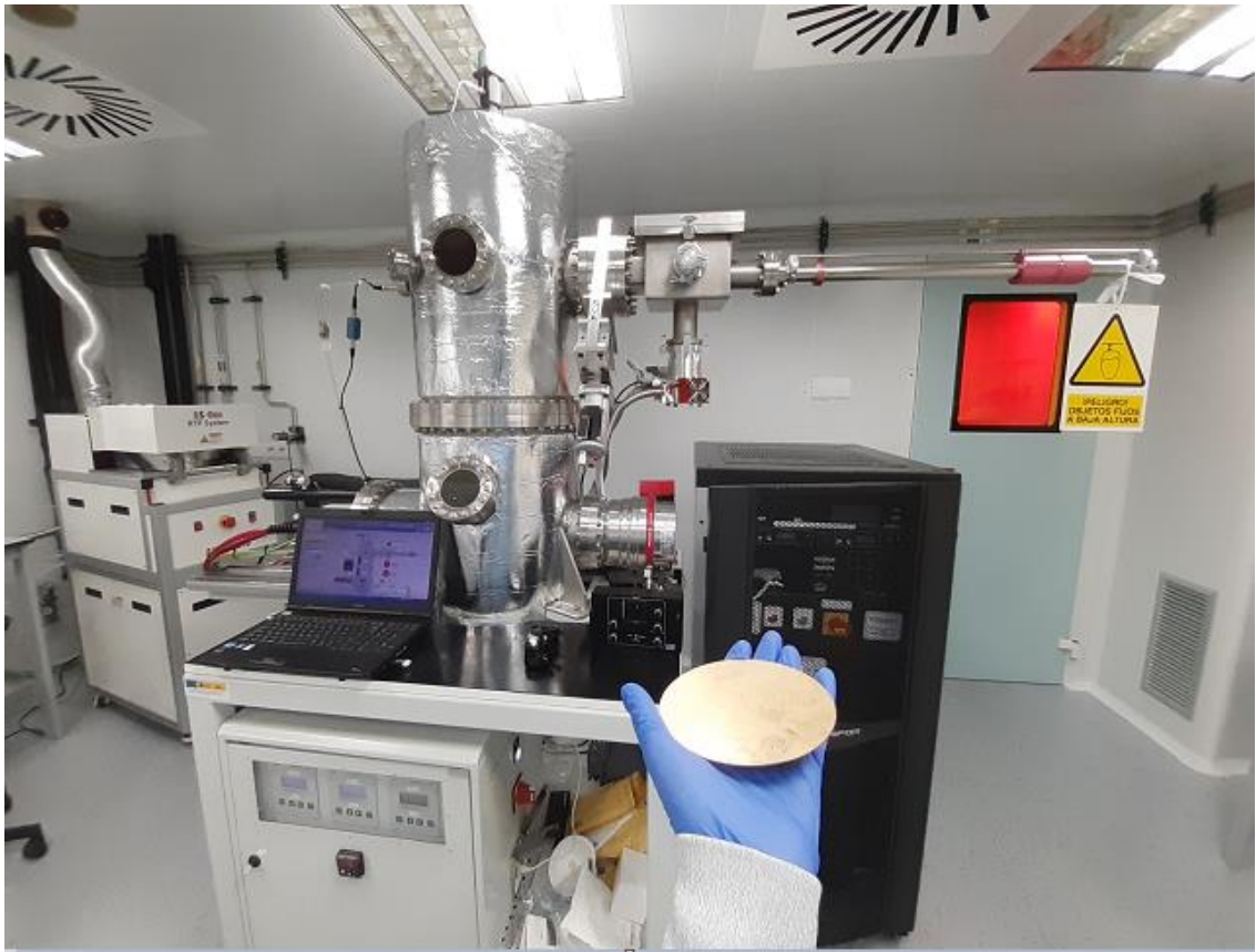
Figure 16: The e-beam evaporator set-up in the cleanroom of the university of Salamanca. The substrate is adhered by Kapton tapes to the wafer shown in the figure and placed in the load-lock chamber. With the help of displacer, it is directed to the evaporation chamber during the process.
