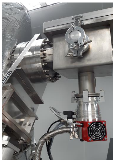
Figure 7: A vertical turbomolecular pump connected to the load-lock of the e-beam evaporator.
