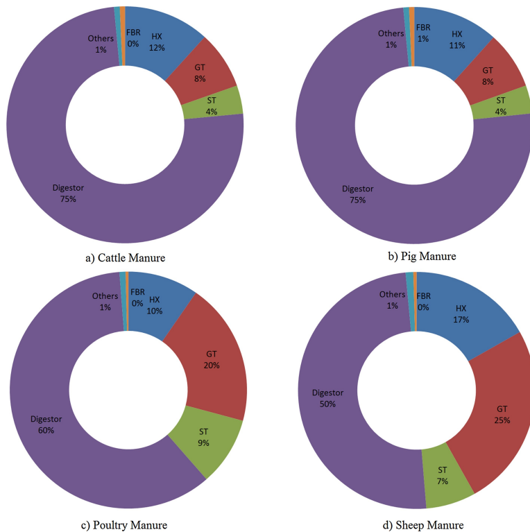
Figure 3.7: Units cost distributions for cattle, pig, poultry and sheep manure treatment (ST: steam turbine, GT: gas turbine, HX: heat exchangers, FBR: fluidized bed reactor).
