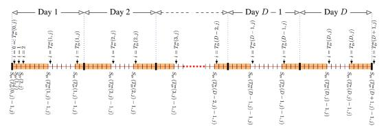
Figure 1. Visualizing the exit and arrival times for j-th EV and the relevance parameters
