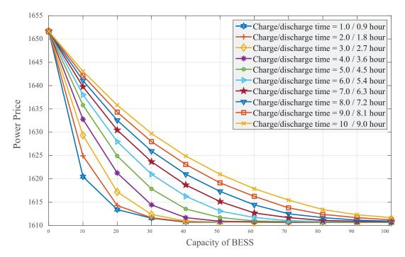
Figure 6. The power price of SB for based on various values of BESS capacity and charge/discharge rate
