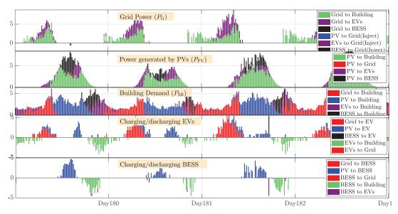
Figure 5. [Scenario 3, days 180 to 183]: Trace of power between Grid, Building's apartments, Pvs, EVs and BESS
